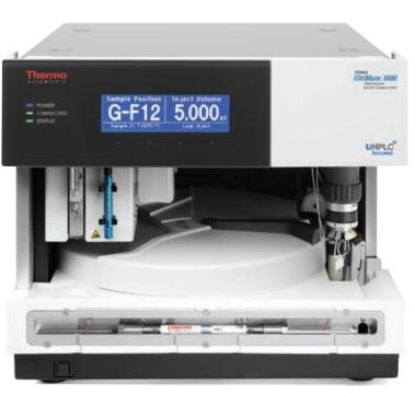
ACC-3000 Autosampler Column Compartment. An integrated column oven provides fast and stable column thermostatting between 5 °C above ambient temperature and 50 °C.
