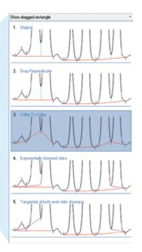
SmartPeaks alternative integration approaches and automatically adds parameters to the processing method for the chosen approach.
