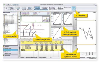
SmartLink displays only data relevant to the current zoom or selected components/injections for fast, easy data evaluation, saving valuable time.
