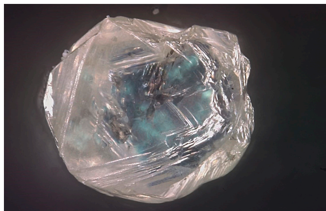
Fig.10: Multifocus image of a raw diamond with transmitted polarized light.
