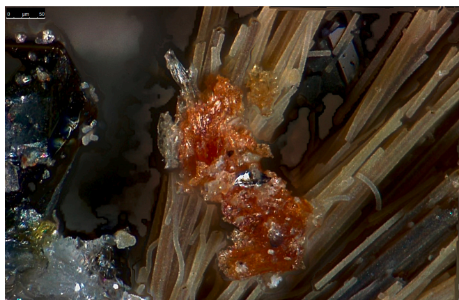
Fig.9: Multifocus image of a micro-mount sample with ring light illumination.
