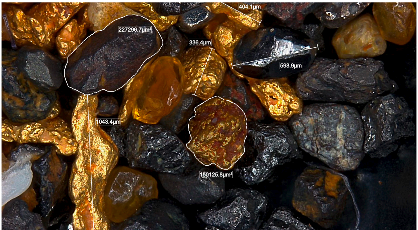
Fig.11: Multifocus image of gold and heavy minerals with length and surface measurements.
