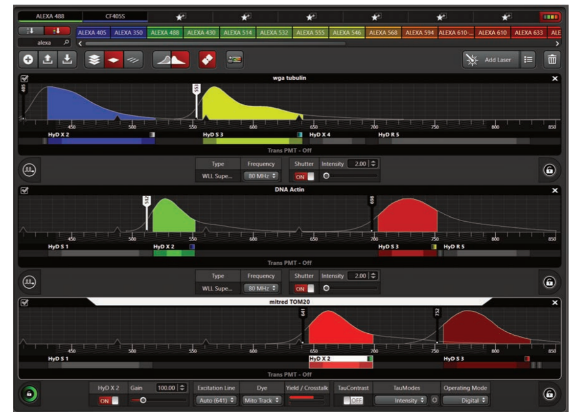
ImageCompass smart user interface. Set up of a 6-color experiment.
