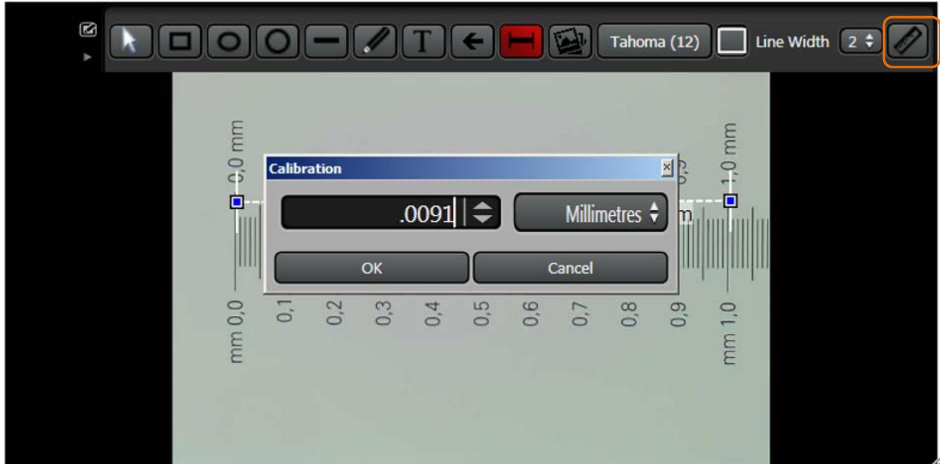
Click the Calibration icon and input the calibration factor. For decimals, start with a “0” before the decimal point. Then select units of measure and click “OK”.
