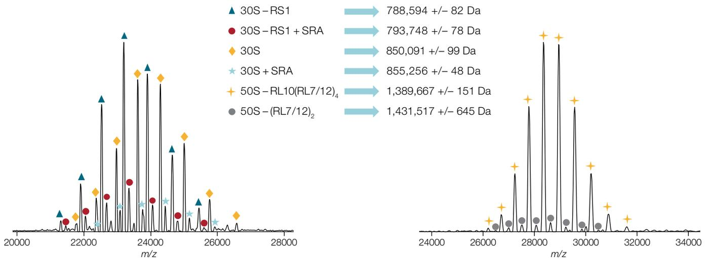
High-resolution MS data produced by the Q Exactive UHMR mass spectrometer reveals the heterogeneity of the ribosomal particles and the substoichiometric association of stationary phase-induced ribosomal-associated protein (SRA).
