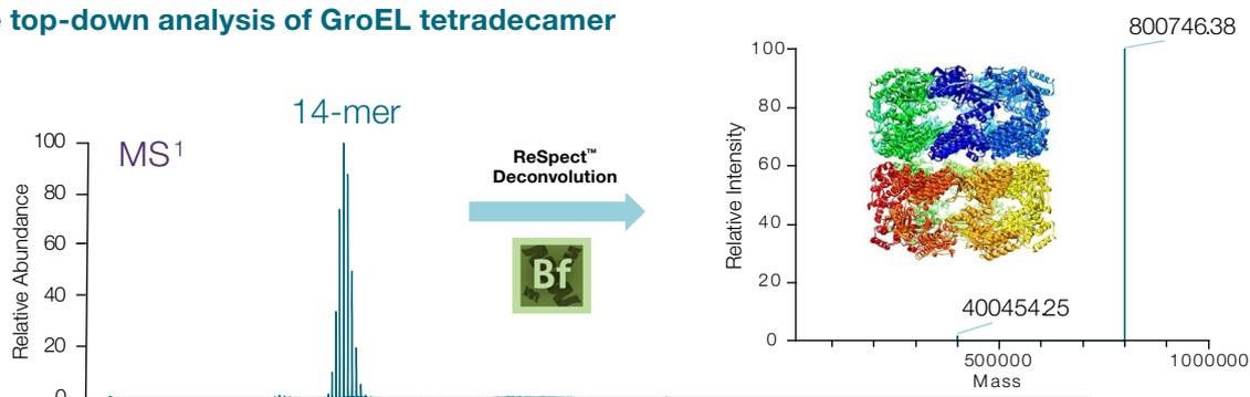
Native MS<sup>1</sup> analysis of the GroEL tetradecamer protein complex, a molecular chaperone required for the proper folding of many proteins in cells. Using in-source trapping, very efficient desolvation and fragmentation of the GroEL 14-mer into monomer and stripped complexes (13-mer and 12-mer) is achieved.
