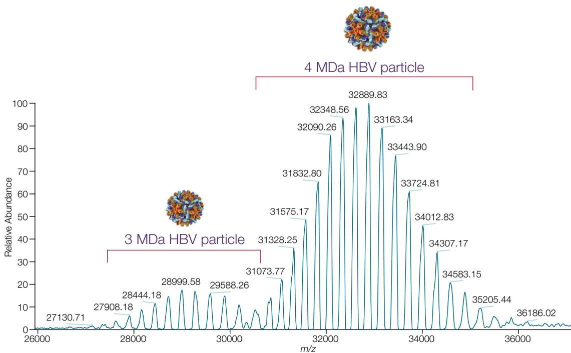
Mixtures of 3 MDa and 4 MDa hepatitis B virus capsids analyzed under charge reducing conditions span a wide mass range between 27,000 and 36,000  $m/z$ . The spectrum contains well-resolved charge states for both particles and shows no bias for the 25% smaller 3 MDa particle.
