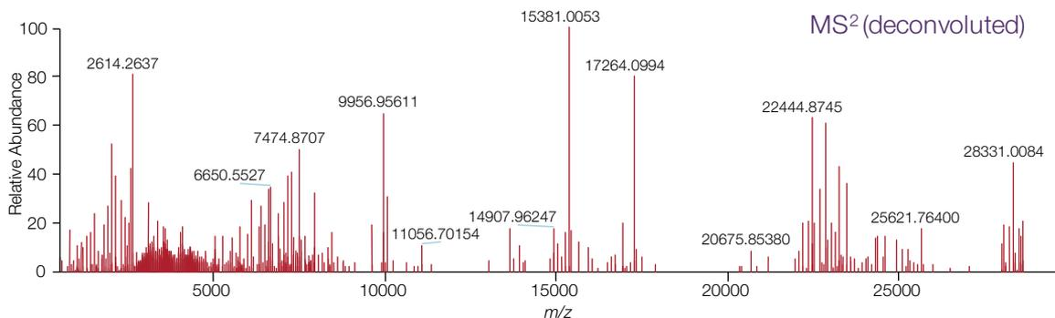
Native top-down analysis of the AmtB membrane protein complex enabled by high mass quadrupole selection and efficient HCD fragmentation.
