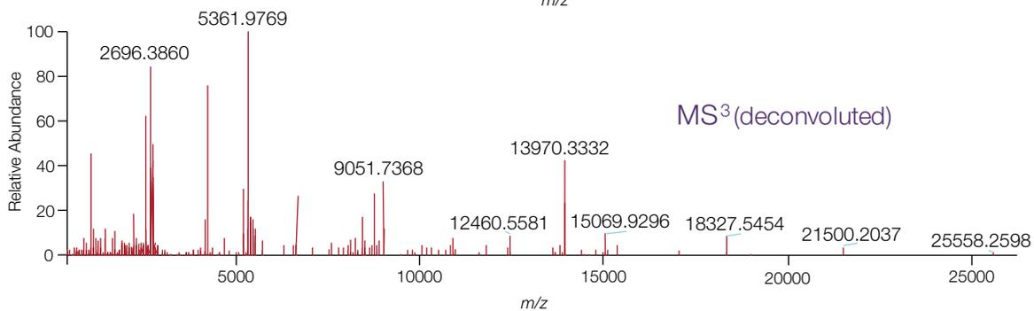
Q Exactive UHMR quadrupole selection of the monomer (shown at the bottom of the previous page), followed by fragmentation in the HCD cell for pseudo-MS<sup>3</sup> analysis.
