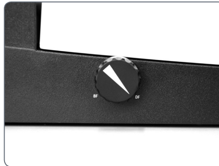
Button to toggle between bright field and dark field
