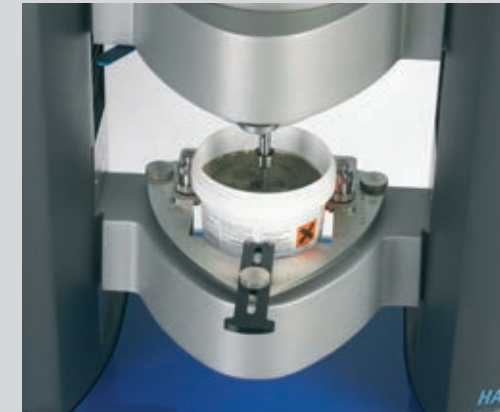
HAAKE MARS equipped with universal container holder for relative tests
