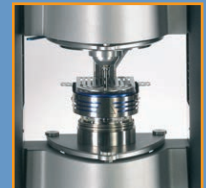
Electrical temperature module for parallel plates with active upper heater
