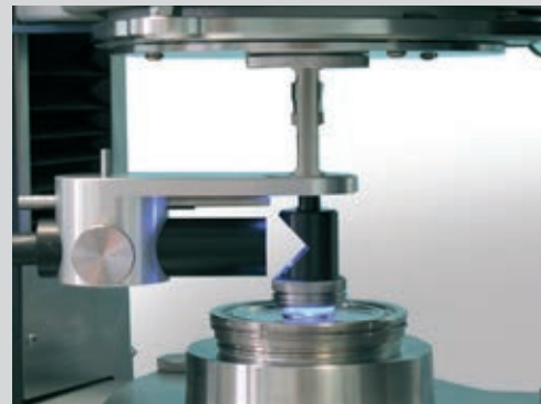
UV curing cell
