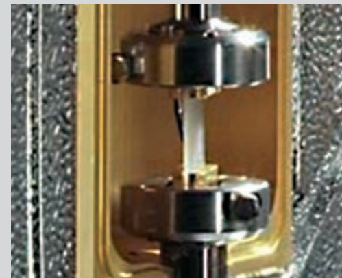
Solid clamps for DMTA on a solid bar
