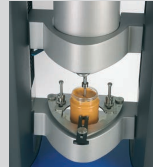
Peanut butter measured with HAAKE MARS, universal container holder and vane rotor
