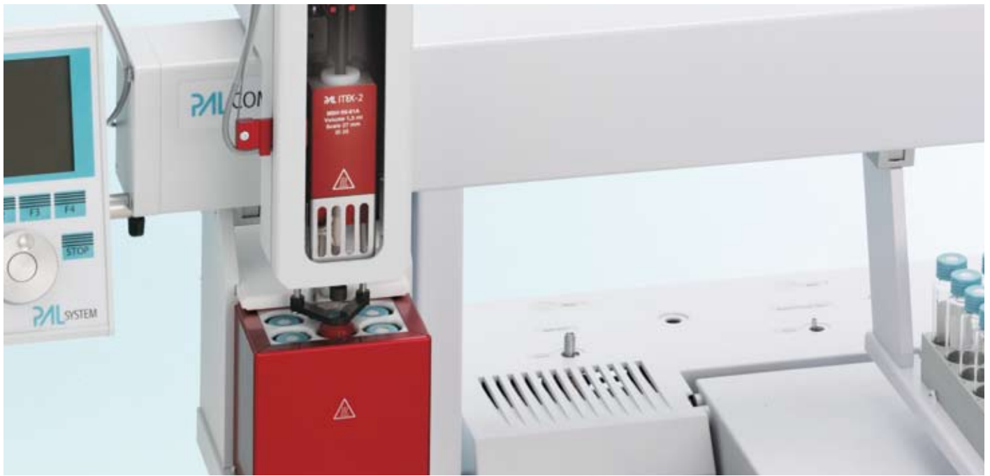
ITEX adsorption step out of a sample vial
