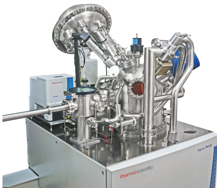
Multi-modal XPS-Raman system, comprised of an iXR spectrometer interfaced to a Thermo Scientific™ Theta Probe X-Ray Photoelectron spectrometer
