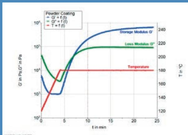
**Investigation of the curing behavior of a powder coating.** The test was performed with a 20 mm parallel plate measuring geometry and electrical upper and lower temperature control modules.
