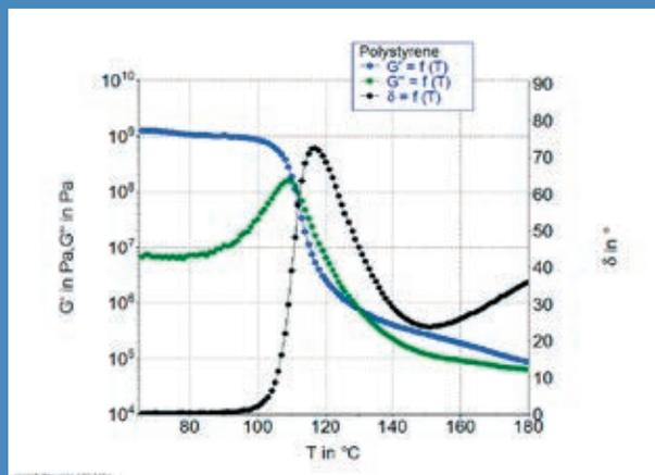
**Dynamic Mechanical Thermal Analysis (DMTA) of a polystyrene.** The test was performed with 8 mm parallel plates measuring geometry and the Controlled Temperature Test Chamber (CTC).
