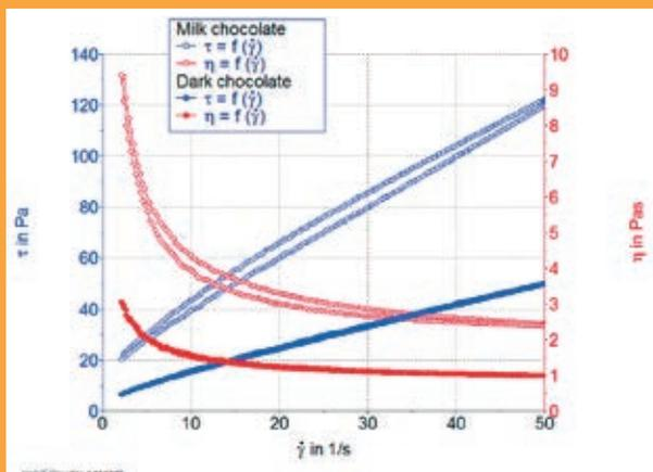
**Rheological test of two different chocolate melts according to ICA method 46.** The tests were performed with a CC25 DIN coaxial cylinder measuring geometry and a Peltier temperature control module.
