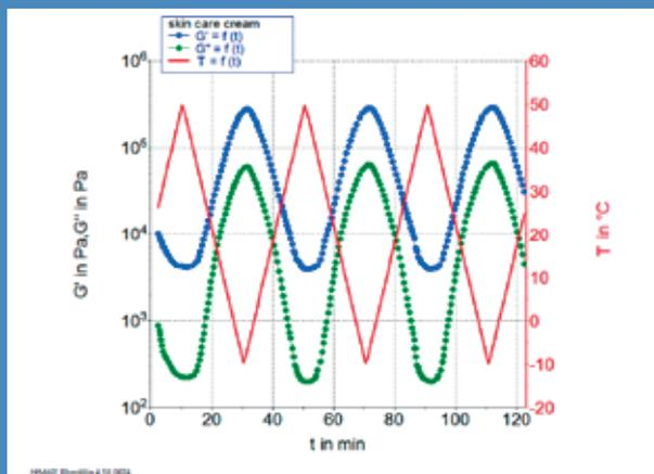
**Rheological swing test to predict the temperature stability of cosmetic emulsions** (Brummer et al.\*). The test was performed with a 20 mm serrated parallel plate measuring geometry and a peltier temperature control module in combination with an insulated sample cover.
