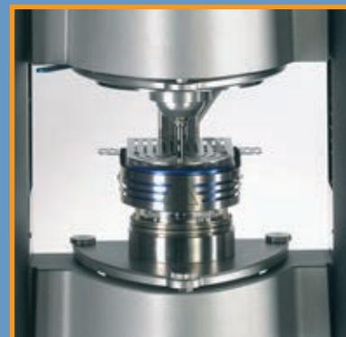
Electrical temperature module for parallel plates with active upper heater
