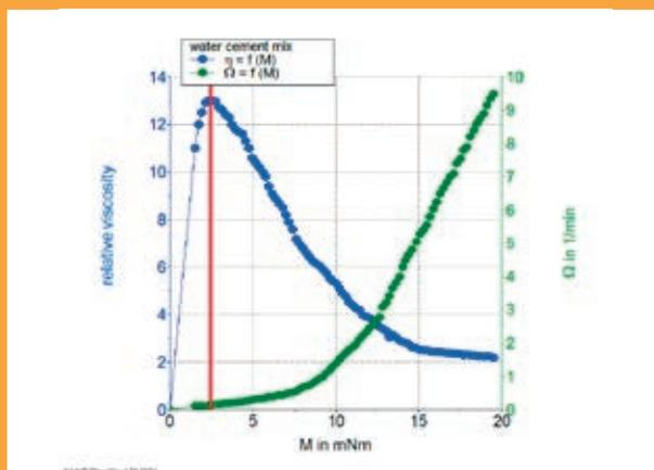
**Determination of yield stress in Controlled Stress (CS) mode of a cementitious paste.** For the measurement the HAAKE MARS was equipped with the measuring cell for building materials and a FL26 CMC vane type rotor.
